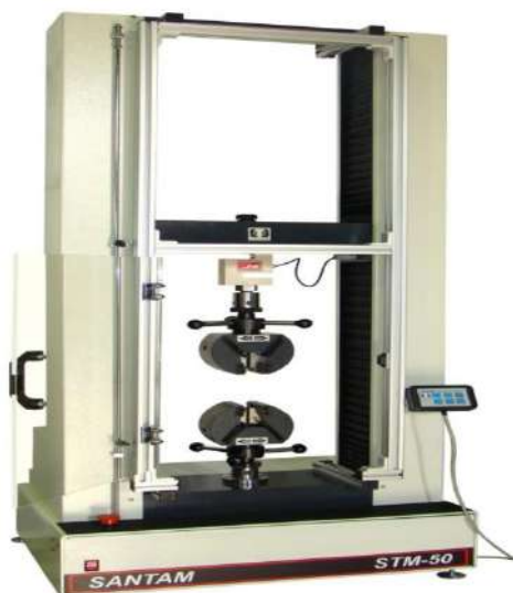
Figure 1. Steel reinforcement bar tensile experimental machine
