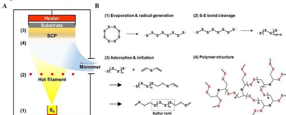
Scheme 7. Sulfur vapor is co-polymerized to form a thin film with a high refractive index.
