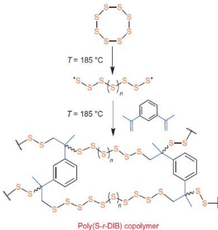
Scheme 3. The production of poly(*S-r*-DIB) co-polymer using DIB cross-linker
