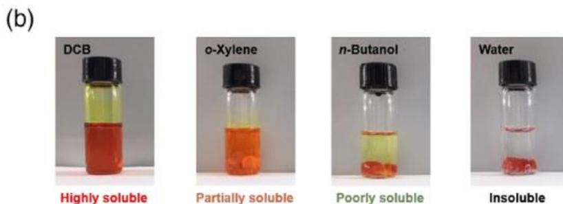
Scheme 6. Solubility test of sulfur-polymer coating. (a) Solution-based sulfur-polymer deposition on planar silicon for film characterization and electrospun Nano fibrillary films for mercury ion removal (left). b) Images of four sulfur-polymer solutions: DCB, o-xylene, and butanol (water).
